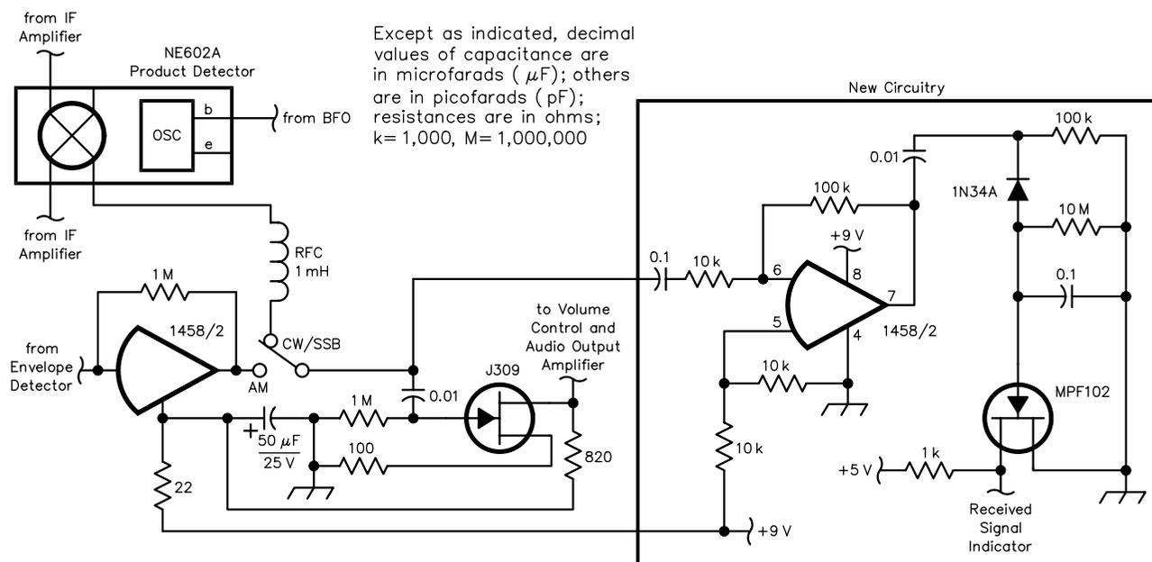
Fig 3—Received-signal indicator circuit.
