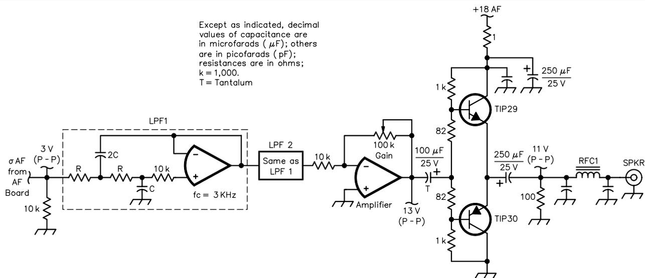
Except as indicated, decimal values of capacitance are in microfarads (μF); others are in picofarads (pF); resistances are in ohms; k = 1,000. T = Tantalum
