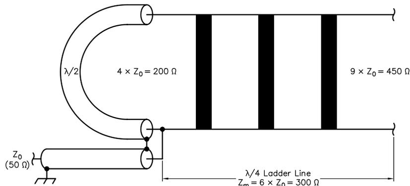
Fig 3—A 9:1 balun using  $\lambda/2$  of coax and a 300-Ω  $\lambda/4$  matching section.
