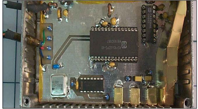
**Fig 11**—All major circuit blocks in the source are designed to be mounted in low-cost, die-cast enclosures from Jameco. Here is a view of a completed NCO board with some added shielding (on the right side) around the 10.7-MHz filter to reduce any clock feed-through to the 10.7 MHz PLL reference signal.
