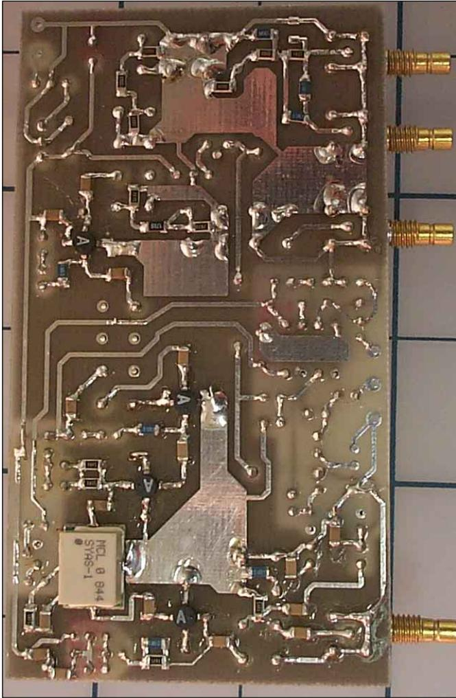
**Fig 10**—The SMT components are attached to the solder side of the PC boards. This is a view of the Mixer board solder side showing SMT construction.
