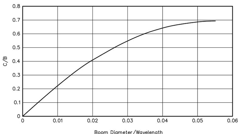
Fig 1—Plot of G3SEK's formula for boom correction.
