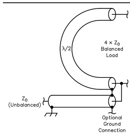
Fig 1—A 4:1 balun using  $\lambda/2$  of coax.
