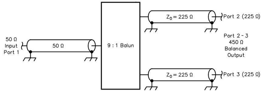
**Fig 4—Modeling a 450-Ω balanced line as two 225-Ω coaxial lines with ARD's three-port model.**
