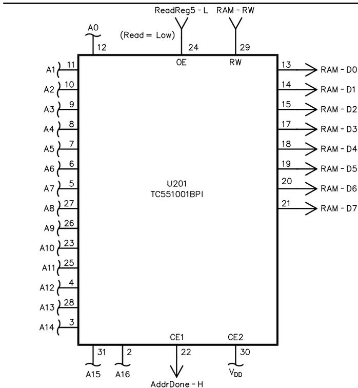
Fig 6—RAM circuit schematic diagram.
