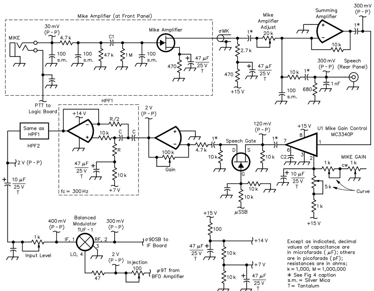
**Fig 9—Transmitter AF-circuit schematic diagram.** For general notes on the schematics, refer to the caption for [Fig 3](#). The signal levels after the mike-gain attenuator are given for the normal control-knob position of 11 o'clock (see Part 1, p 21 for information about microphone calibration). The DBM used as a balanced modulator may be obtained in small quantities directly from Mini Circuits.
