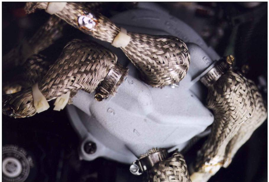
Fig 1—Braid installed over spark-plug wires at distributor.
