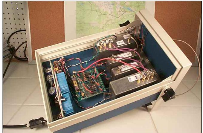
**Fig 12**—What all your hard work can produce—your own VHF synthesized source. I used a new Bud chassis to house my source, but a surplus enclosure can work equally well.
