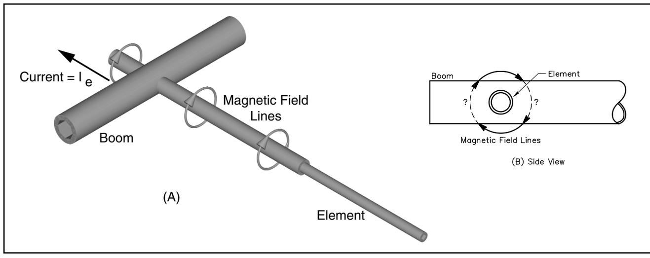
correction  $C$  for any combination of boom diameter, element diameter and element length. This involves using *YO6*, first to find the complex impedance  $Z$  of the uncorrected element length and hence its phase  $\phi$ . Then by a process of trial and error to find a new element length which, when combined with the negative reactance contributed by the boom, has the same phase.
