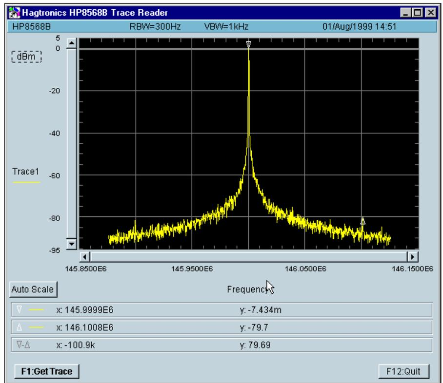
Fig 8—The close-in spurious performance of the source shows a reference rejection of -80 dBc. The span for this display is ±125 kHz from the carrier.
