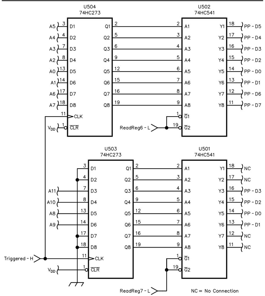
Fig 5—Pre-trigger circuit schematic diagram.
