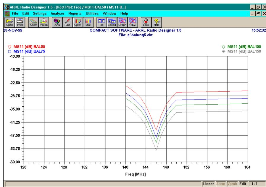
Figure 2—Raising the coax impedance to from 50 to 150 Ω improves the bandwidth of a 50:200 Ω  $\lambda/2$  coaxial balun.
