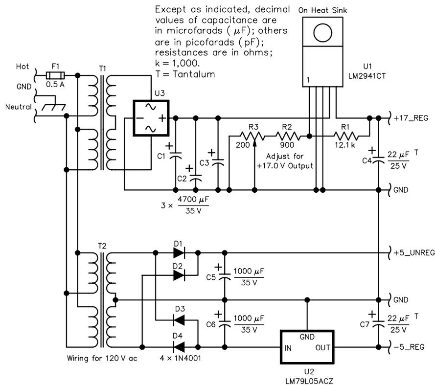
**Fig 6**—The power supply uses toroidal transformers to prevent radiated magnetic fields from modulating the source output. As a further noise-reduction technique, all of the critical RF modules contain their own local linear voltage regulators to prevent cross-talk. Unless otherwise specified, use 1/4 W, 1%-tolerance carbon composition or film resistors.
