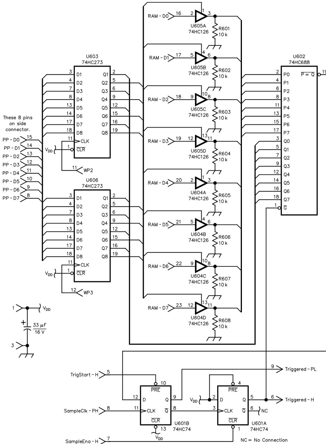
Fig 8—Trigger circuit schematic diagram.
