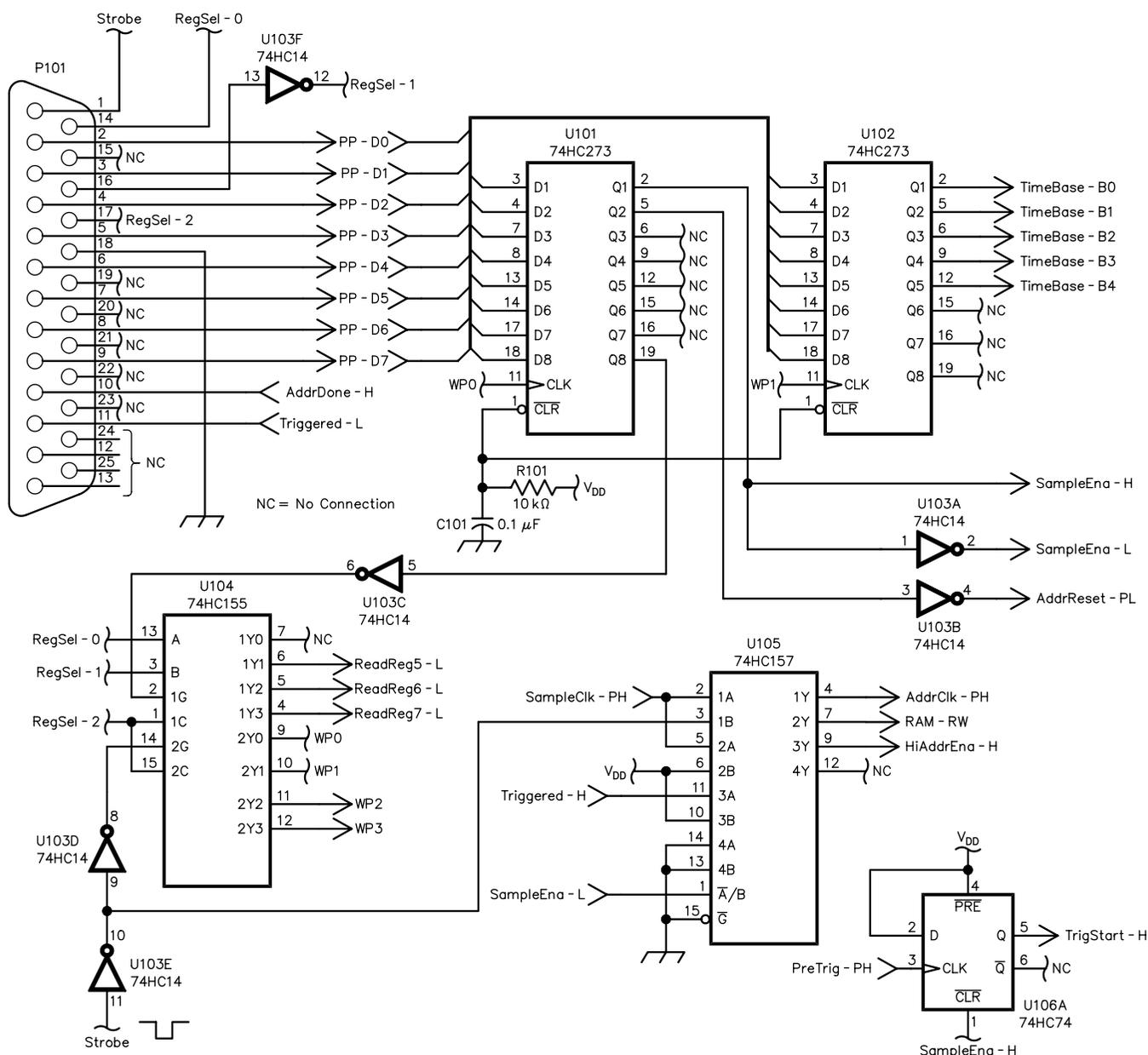
Fig 3—Control circuit schematic diagram.
