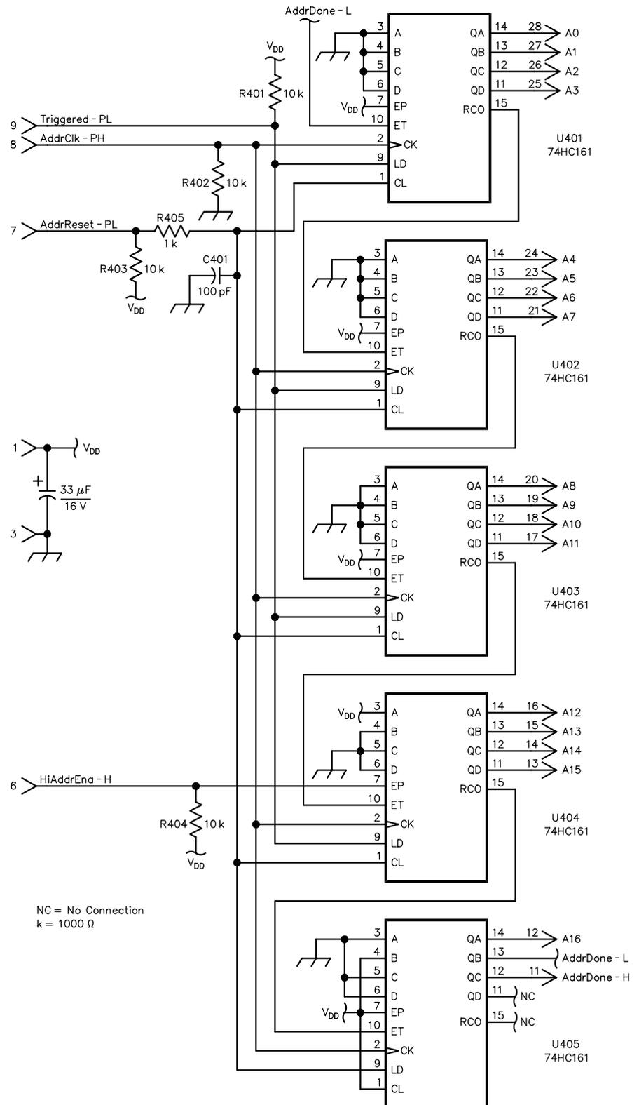
Fig 2—Address Generator schematic diagram.
