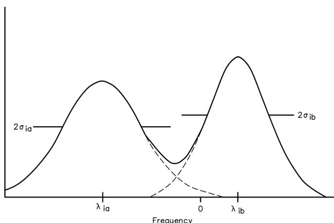
Fig 2—Tap-gain distributions for a two-ray model.
