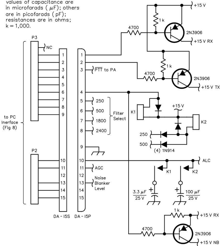
Fig 9—Transceiver control circuits. Unless otherwise specified, use  $1/4$  W, 5%-tolerance carbon composition or film resistors.
