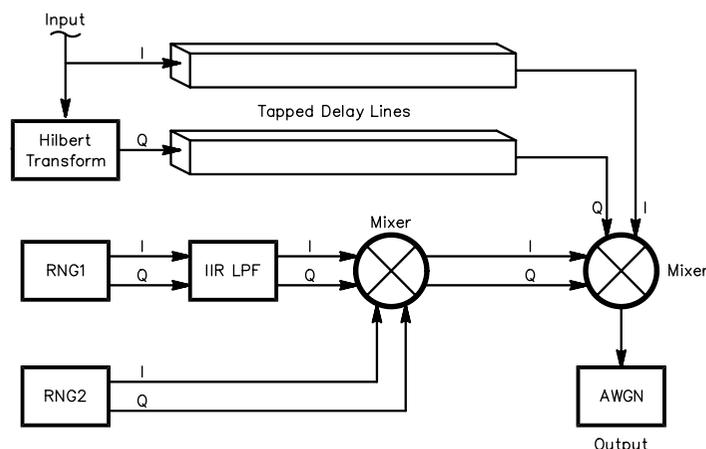
Fig 3—Simulator process flow.
