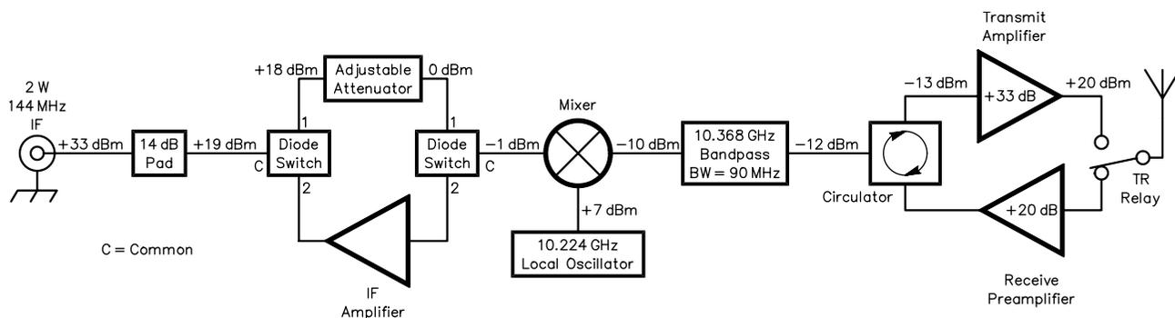
**Fig 2—Block diagram of a 10 GHz transverter using a circulator and surplus parts. The power levels in dBm are typical transmit levels.**
