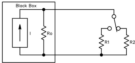
Fig 1—Load-pull method to find value of  $R_o$ .
