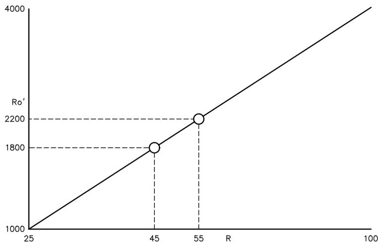
Fig 3—Variation of  $R_o'$  versus  $R$  for a conventional transformer.
