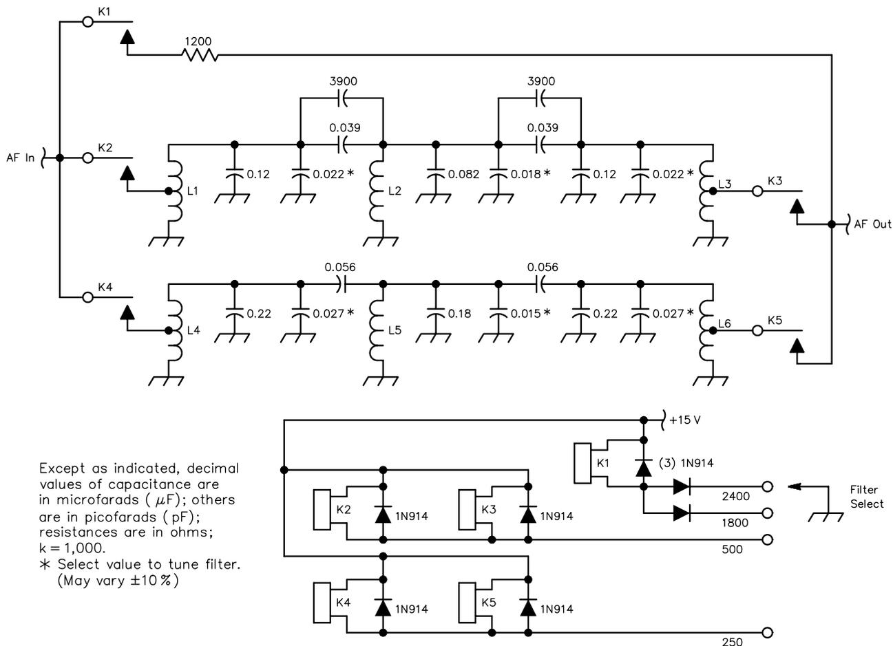
**Fig 5—AF filter schematic diagram. Unless otherwise specified, use  $\frac{1}{4}$  W, 5%-tolerance carbon composition or film resistors. All capacitors are  $\pm 5\%$  tolerance mylar components.**
