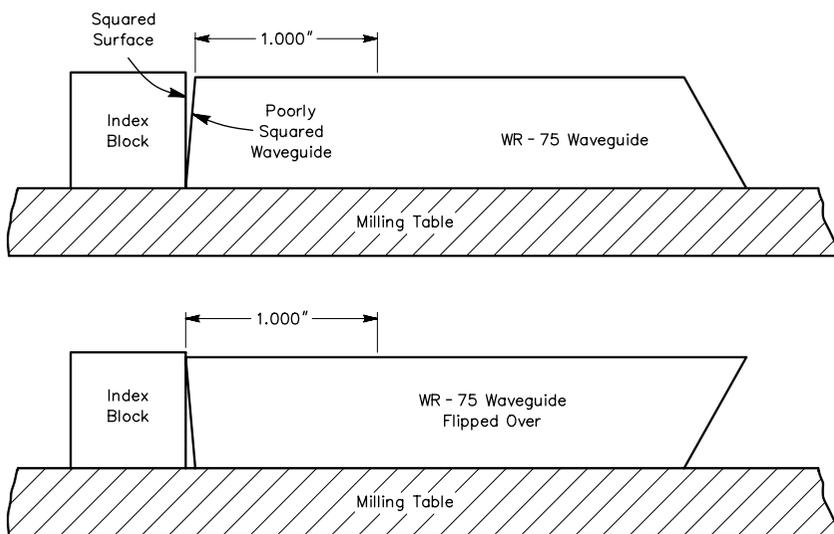
Fig 3—The use of an index block with a squared surface preserves milling-machine accuracy despite the imperfect waveguide end when the waveguide is flipped over to drill matching holes on the opposite side.
