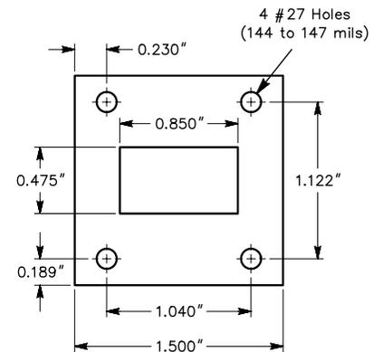
Fig 4—Homebrew WR-75 flanges made from 0.032-inch-thick brass sheet.
