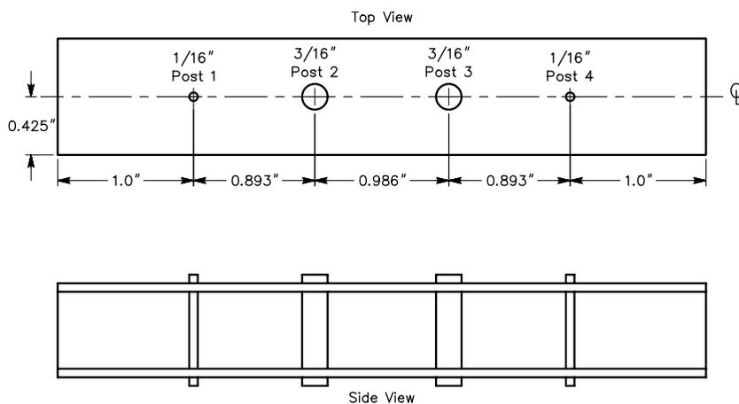
**Fig 1—Construction details of the WR-75 filter. Posts 1 and 4 are  $\frac{1}{16}$ -inch brass rod. Posts 2 and 3 are  $\frac{3}{16}$ -inch brass tubing; the wall thickness isn't important. The waveguide is 4.8 inches of WR-75.**
