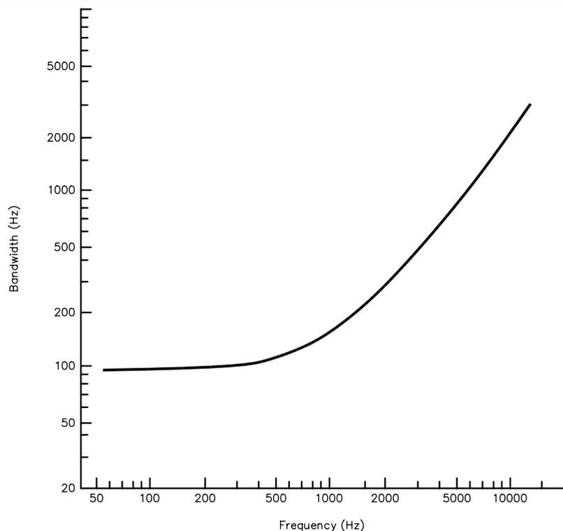
Fig 2—Critical BW versus frequency.
