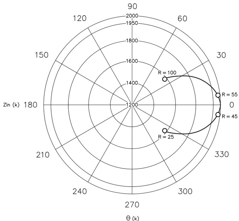
Fig 5—Input impedance and phase of the Pi network as a function of output load resistor  $R$ .
