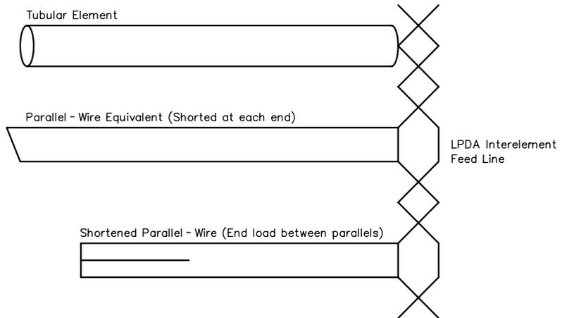
Fig 18—Evolution from tubular elements to equivalent wire elements to possible shortened-wire elements.
