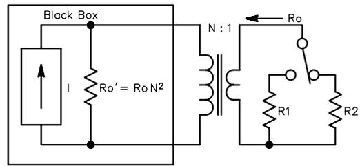
Fig 2—Finding  $R_o$  when a transformer is in the circuit.
