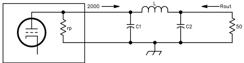
Fig 4—Pi network from tube to 50  $\Omega$  load.
