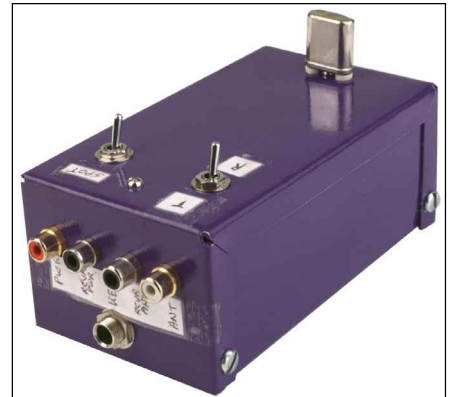
On the rear panel of the 10-meter transmitter, four phono jacks provide connection to the power supply (PWR), receiver (RCVR PWR and RCVR ANT) and the station antenna (ANT). A 1/4-inch KEY jack is beneath the phono connectors. The receiver/transmit (R/T) and SPOT toggle switches are at the rear of the top panel, with the crystal socket toward the enclosure's front.
