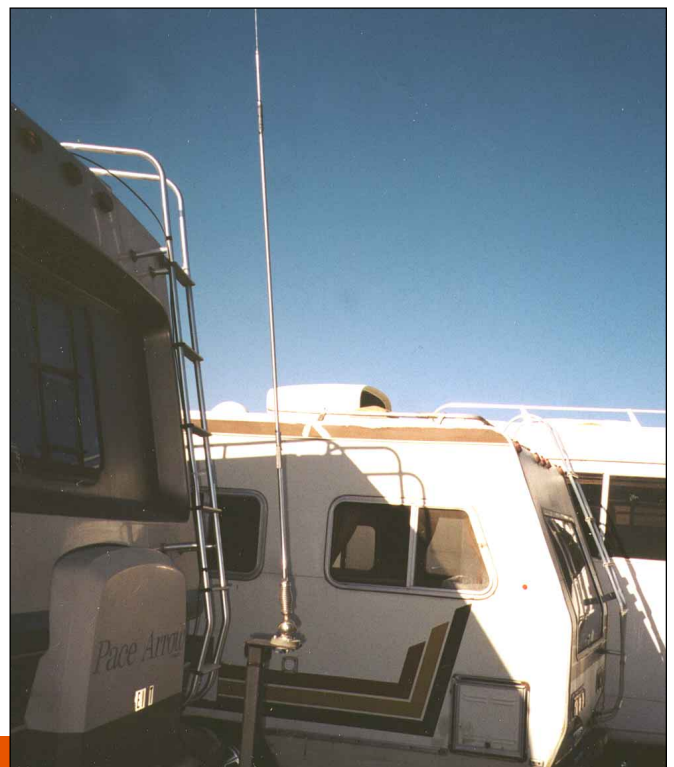
Talk about a rugged antenna mount! Lewis, W7JCV (left), crafted this motor home antenna mount with the skilled use of a welding torch. Not only is the mount strong enough to keep his tall whip antenna in place (right), it is also removable.
