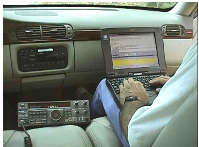
The author pulls over at a promising location, switches on his transceiver, opens his laptop computer and works PSK31.
