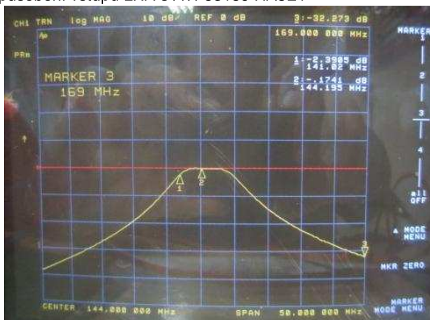
obr.č.5 Zisk LNA s ATF53189 HA8ET
